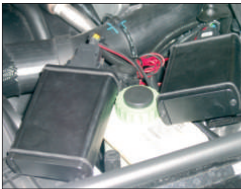
Twin Tunit boxes for the twin ECUs.
